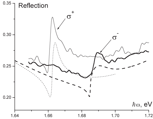
Figure 5. Normal incidence reflectance spectra for \sigma^+ - (thin solid line) and \sigma^- -components (thick solid line) of the exciton band of the 18 ML-wide QW with magnetic ions content x = 0.014 . The measurements were carried out at T = 2 K in the magnetic field B = 3.2 T. Corresponding calculated curves are plotted using thin and thick dashed lines, respectively, \hbar\Gamma_0 = 1.1 meV).
